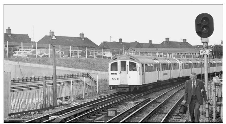
Above: The old terminus at Hounslow West with a Piccadilly Line train of 1959 Tube Stock arriving. By this time the third platform had been decommissioned to make way for the forthcoming Heathrow extension, the civils work for which can be seen to the left of the train.
